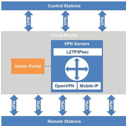
**Cloud Router acts as intermediary between control stations and NetModule Routers in the field. Cloud Router is a software package for Debian Linux.**
