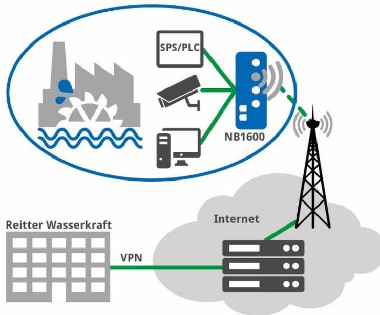
The power stations of Reitter Wasserkraft are monitored in different ways. There are in principle three possibilities: Passive queries of power, temperature or water level via a PLC in the power station, active remote access to the central computer and video surveillance. In addition to these measures, SMS messages are sent via the NB1600 in case of emergency.
